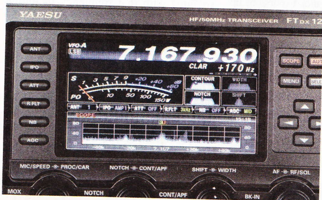
Figure 1 — The colorful LCD shows many operating parameters.
