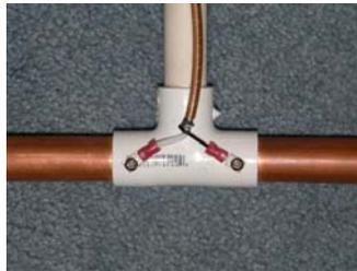
Now its time to make the phasing harness using 75ohm coaxial cable. RG-59 is a convenient size since there are readily available adapters for PL-259 connectors. I have since found type F female T adaptors from L-com and will be using them with RG-6 and compression type F connectors on my next version.
