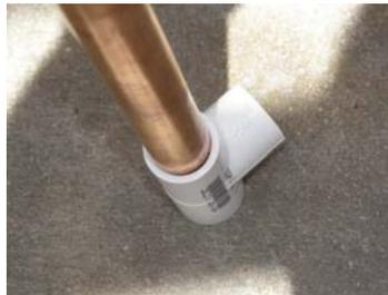
To insert the other half of the dipole element, place previously installed copper pipe side on the hard floor with the PVC T facing upward. It takes a little balancing to hold the joined sections while pounding the second copper pipe in and another set of hands would be helpful. You may have to warm the PVC T again before this step. Make sure the two copper elements are going together concentrically by looking down the side of the pipes as they go together.
